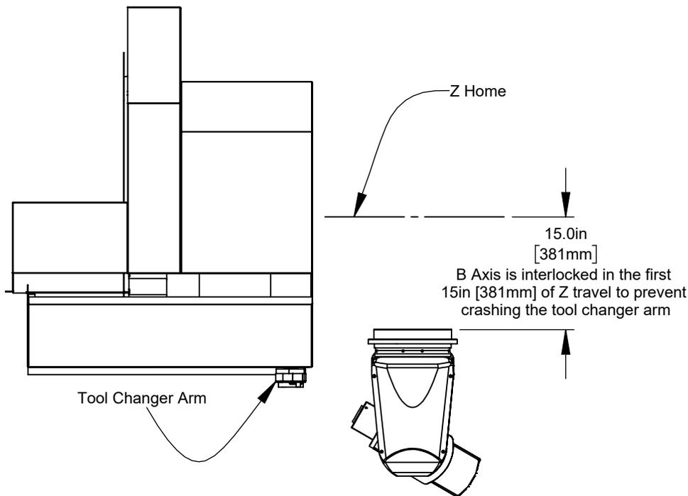
In addition to the tool changer interference zone, the machine has restricted zones between the gimbal head and fixed machine elements
