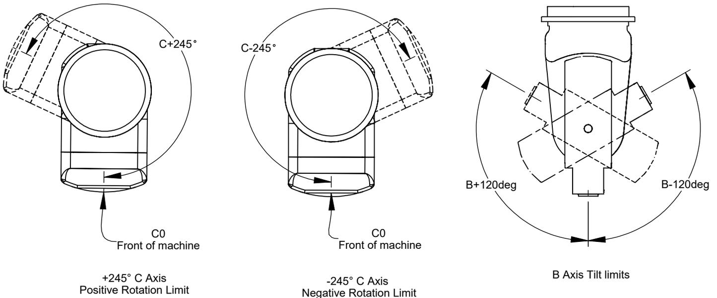
Isometric view of B & C Axis gimbal head for visual reference
