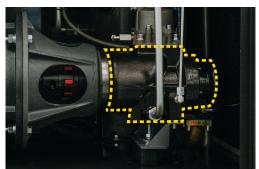
**Rotary-Screw Air Compressor**
