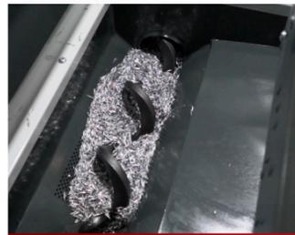
SISTEMA DE PARAFUSO SEM FIM DA LIMALHA
