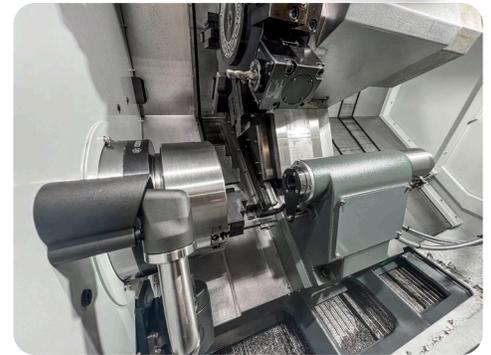
Each SB Series lathe is equipped with a robust 12-station BMT65 turret that accepts industry-standard base-mount tooling, as well as axial and radial driven live tools for secondary milling, drilling, and tapping operations.
