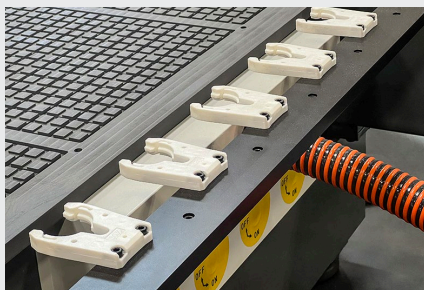
THE SR-3015P FEATURES AN 8-STATION LINEAR TOOL CHANGER FOR OPTIMIZED TOOL CHANGES AND FASTER CYCLE TIMES.
