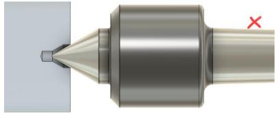
Incorrect drill depths being too shallow or too deep will lead to improper work holding.
