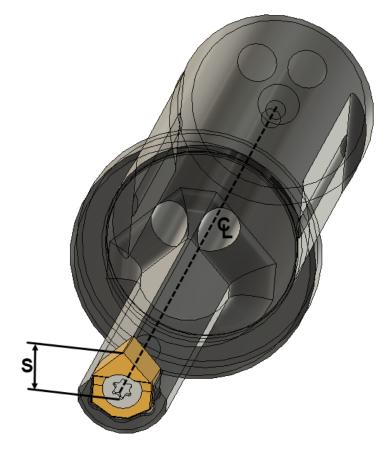
• S dimension is taken from tool holder centerline to the tip of the Haas Square inserts.
