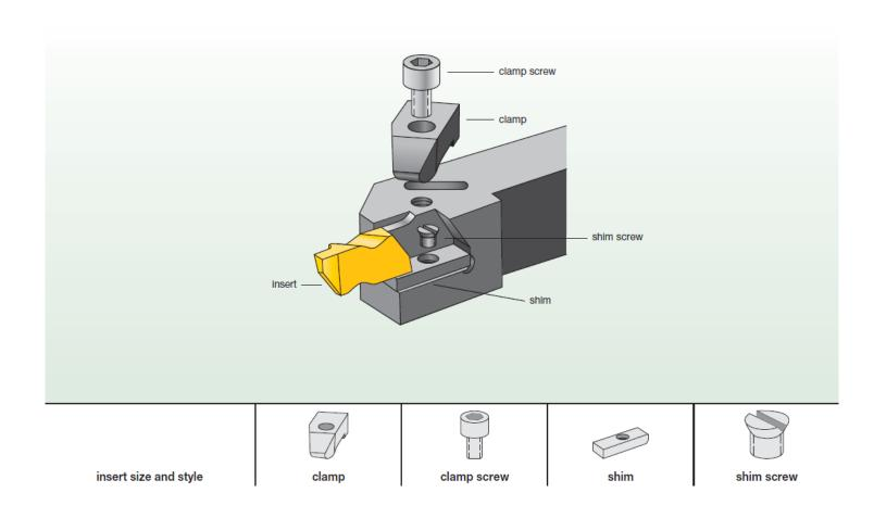
Applies to Both OD and ID tool holders Shim and Shim screw not required for all tool holders. Check related products
