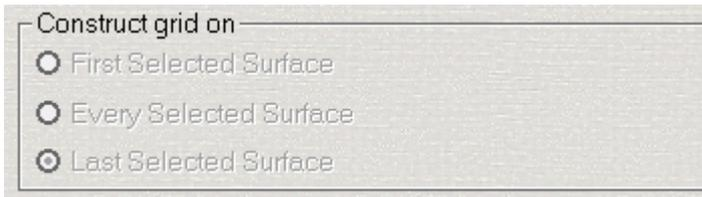
This option will be available once the user selects more than one surface on a CAD model. These options lets the user to determine how the grid points will be distributed on the selected surfaces.
