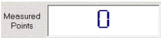
Acts as a point counter when features are in the process of being measured.
