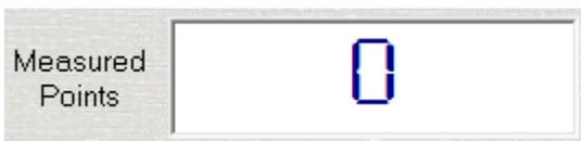
Acts as a point counter when features are in the process of being measured.
