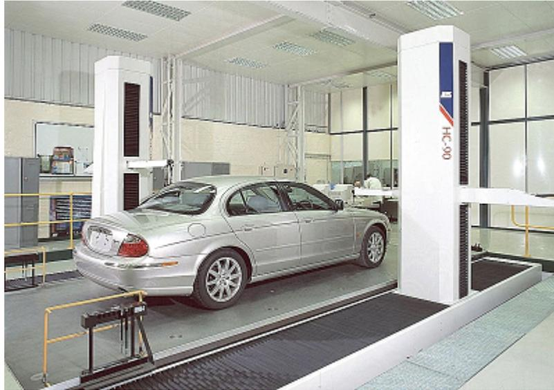
In order to create a single measurement database, where the features measured from each machine are stored and reported, CAPPS configures dual arms as **Master (client) and Slave (server)**. Hence, the data obtained by the server computer is transferred to the master computer for storage and measurement analysis.
