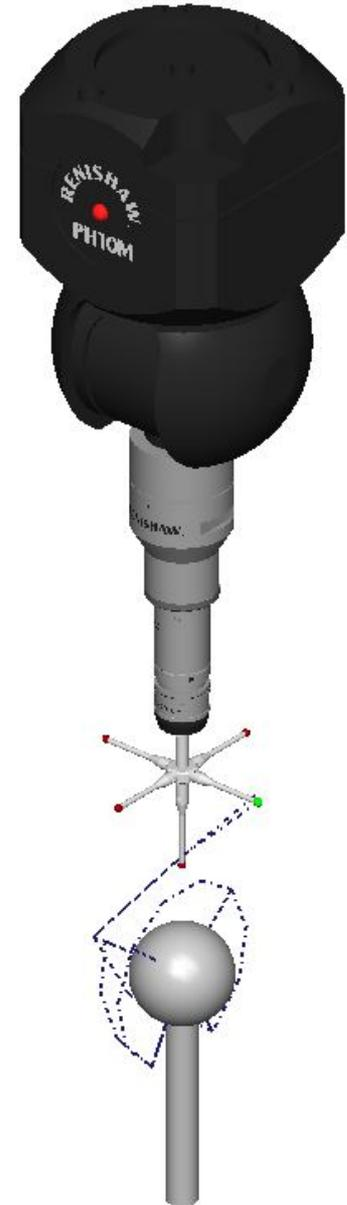
**TIP 4** calibration path with **head angle** at **A=45 B=30** is shown below. Also note that the **Probe Label** automatically adds the head angles to probe label along with the tip number.
