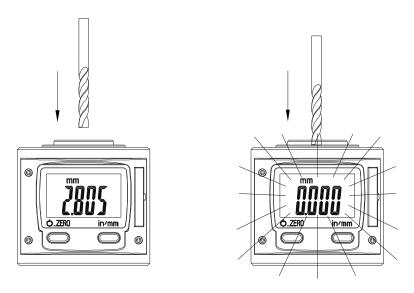
**NOTE:** The height setter will reset to factory settings after 8 hours, requiring the zero point to be reconfigured.
