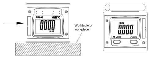
2. Place the bottom end on a ferrous surface to fix the height setter in place. Slowly descend the cutting tool onto the contact surface until the LED display lights up and reaches zero.
