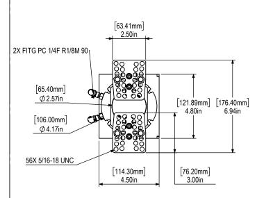
Total weight of the Single Pneumatic Gripper: About 7.5lbs [3.4kg]
