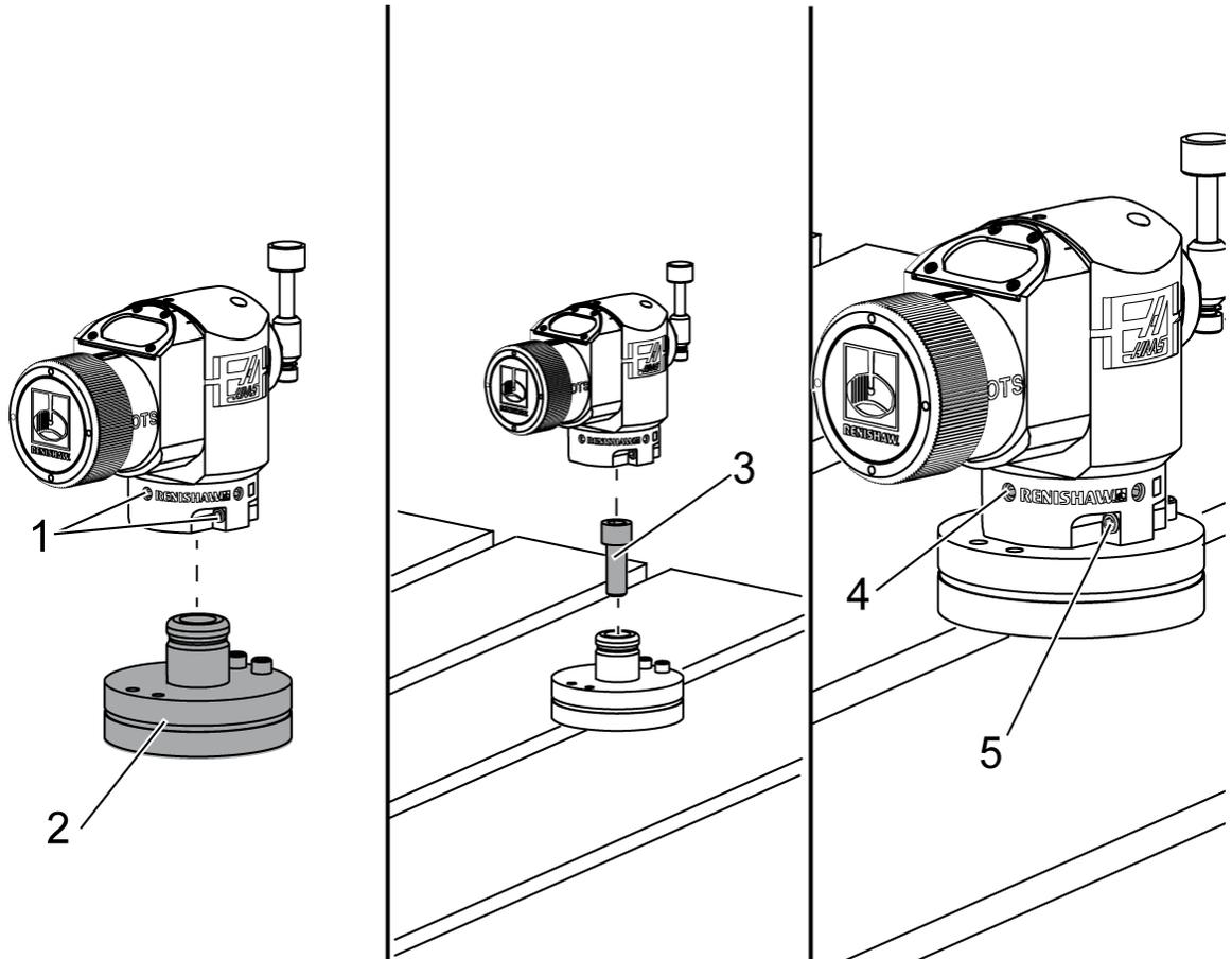
The recommended tool probe location is on the right side of the table, away from the tool changer. This position also allows the probe window to face away from flying chips, prolonging probe life. The spindle must have enough travel to reach all four sides of the probe stylus. Allow 2" of travel on all four sides of the probe stylus, for calibration.
