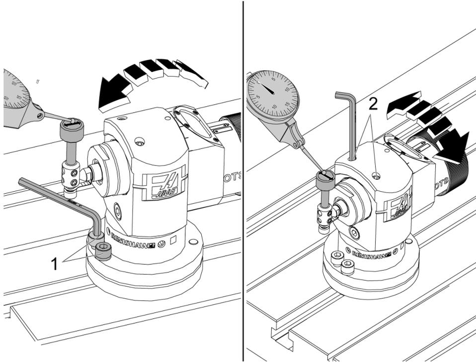
Attach the base of your dial indicator to the spindle and place the indicator tip on the tool probe stylus.
