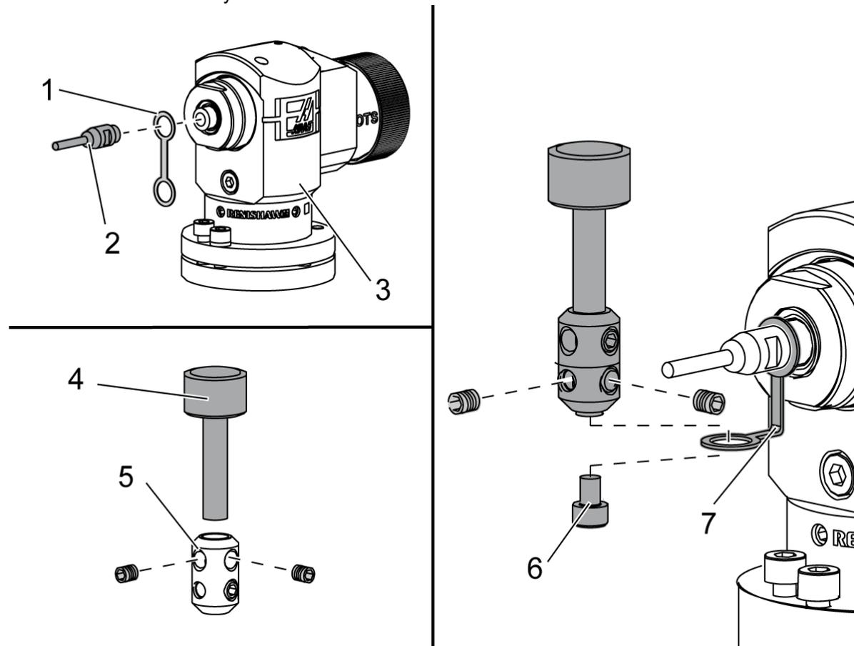
Place the retainer strap [1] over the shaft mount on the probe body [3].
