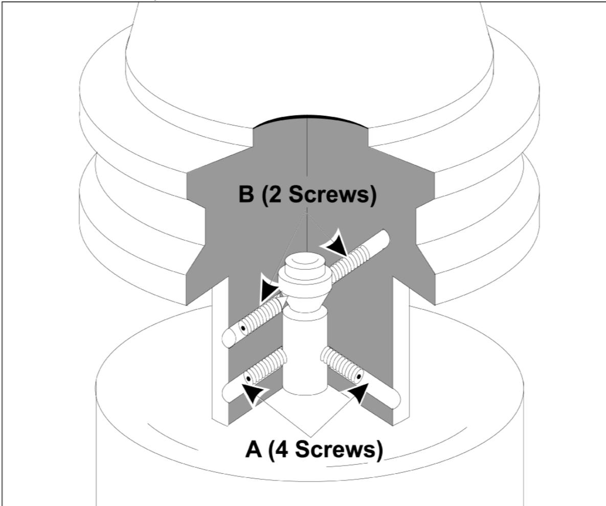
Insert the OMP40-2 probe into the spindle.
