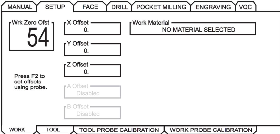
1. Select a Work Coordinate System. Press **[WRITE/ENTER]**.
