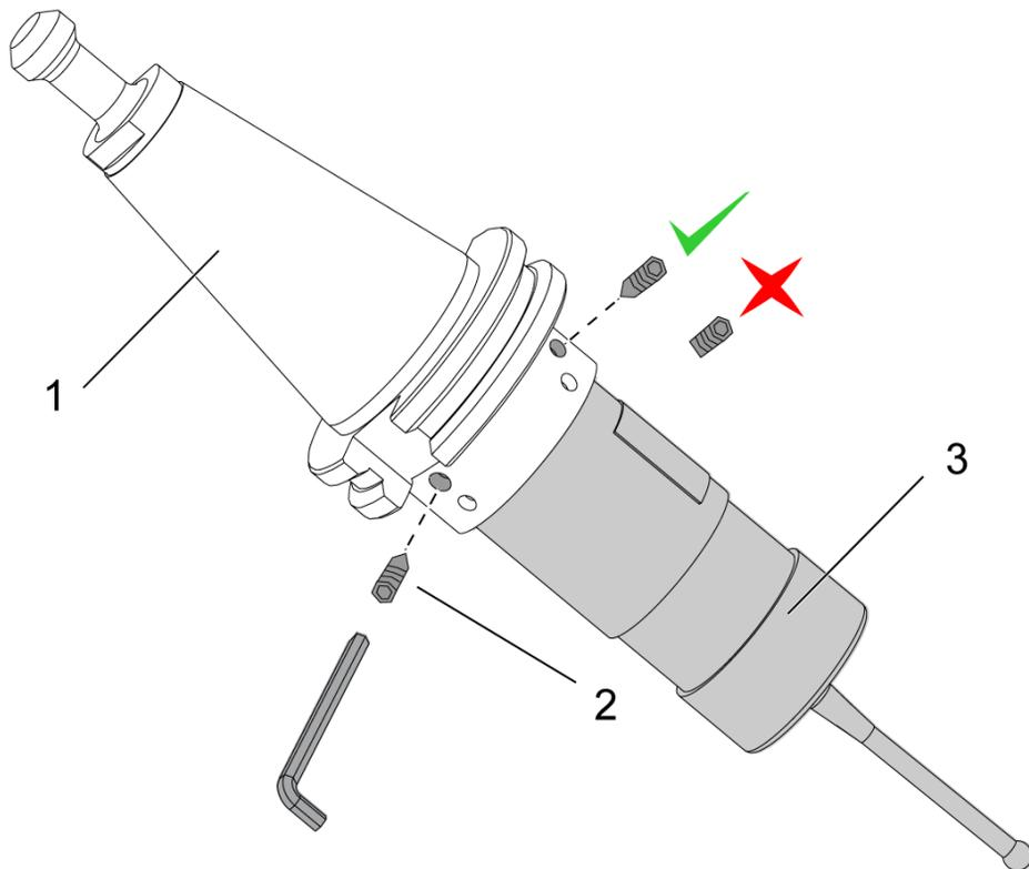
If the probe is not yet installed to the toolholder, follow the below steps, otherwise skip to Step 3:
