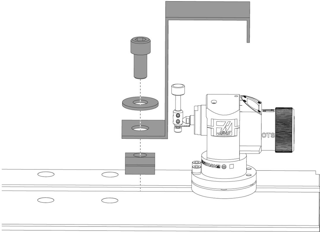
Remove the red shipping bracket and associated mounting hardware.
