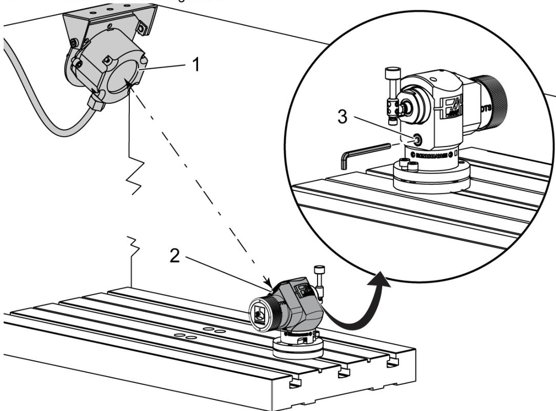
Loosen the set screw [3] beneath the stylus.
