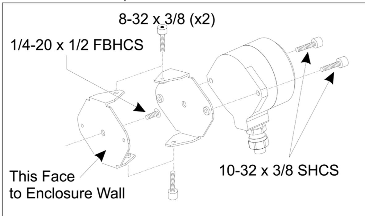
Secure one bracket to the OMI using two 10-32 x 3/8 SHCS.
