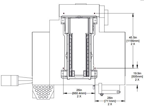
Note: Machine must be placed on one continous concrete slab. Slab should extend 12in [305mm] beyond anchor holes in all directions
