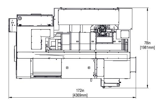
WHEN THE CONVEYOR OPTION IS SELECTED, IT SHIPS IN THIS VERTICAL POSITION
