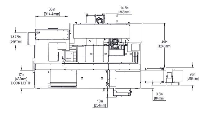
CONVEYOR REMOVAL DISTANCE IS 67in [1702mm]
