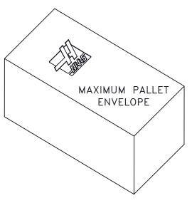
1213mm X 517mm X 508mm LENGTH x WIDTH x HEIGHT (Workholding + Part)
