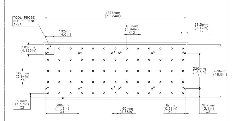
"A" THREADED HOLES ARE FOR FIXTURE PLATES
