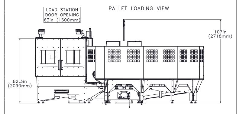
Maintain 3 feet (915 mm) clearance to the nearest obstruction around all sides of machine perimeter for maintenance access
