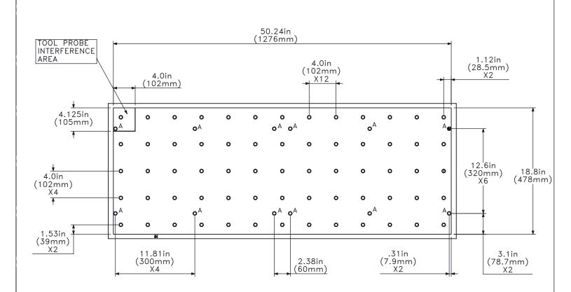
"A" THREADED HOLES ARE FOR FIXTURE PLATES
